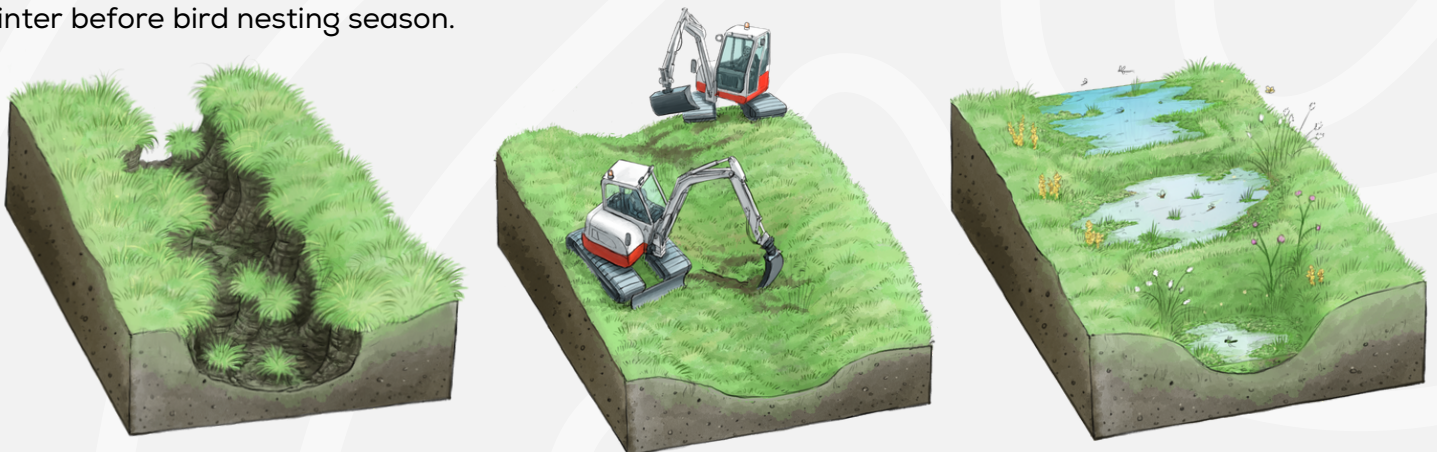
Figure 4 : Illustrations showing the process of reprofiling peat hags and erosion gullies into a shallower gradient, and adding peat bunds, will overtime slow the flow of water and reduce erosion of the exposed peat.
