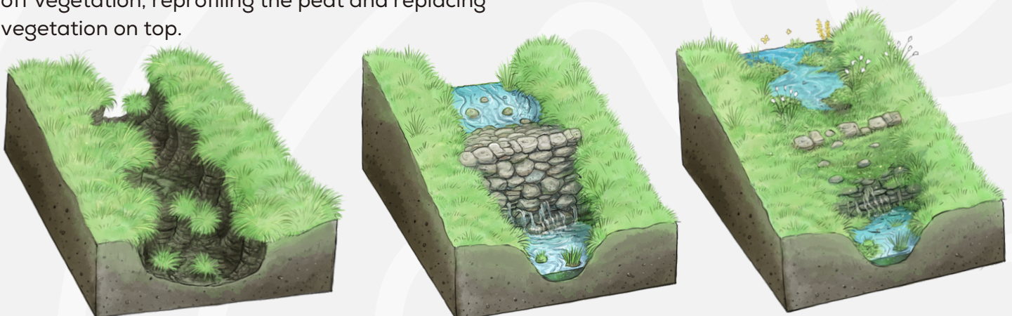
Figure 3 : Illustrations showing the process of blocking erosion gullies with stone to slow the flow of water and reduce erosion of the exposed peat.
