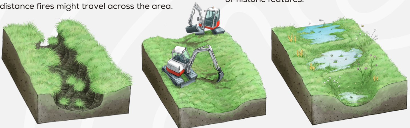
Figure 3 : Illustrations showing the process of reprofiling peat hags and erosion gullies into a shallower gradient, and adding peat bunds, will overtime slow the flow of water and reduce erosion of the exposed peat.
